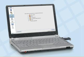
A highly secure platform for processing and storing classified information in mobile and office environments. IPSec VPN, Hard Disc Encryption together with a Smartcard for User Authentication operate independently from the Windows or Linux Operating System. Approval: up to CONFIDENTIAL.
